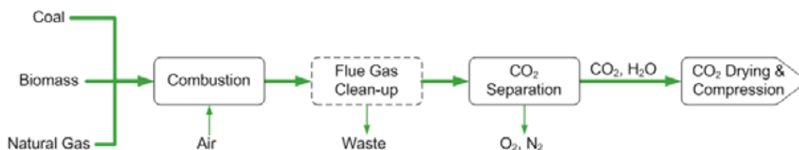
Figure 2.3: A flow diagram showing the flow of carbon in post-combustion CO 2 capture. Flue gas clean-up is only required for solid fuels, as natural gas contains low concentrations of sulfur and combustion can be controlled to minimize the concentration of NO x .
